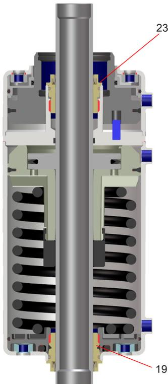
fig. 23: Actuator screw
