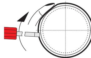
4. Press the seat assembly tool between the seal shoulder and the groove edge (both sides). Proceed around the circumference. Then proceed around the circumference of the lower seal shoulder. This is to vent the seal groove and to lock the seal shoulder.
