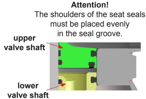
1. Provide the seal shoulder with a thin layer of grease.
