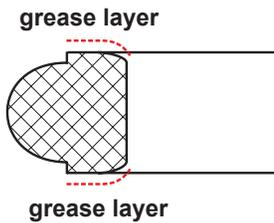
2. Insert the seat seal into the valve shaft, making sure the seal is positioned at an angle, as shown below.
