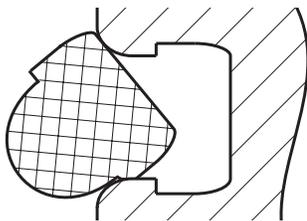
3. Press the seal circumferentially into the groove using the seat assembly tool (part no. 102797+) or a screwdriver with round edges. Place the assembly tool at the upper seal shoulder. To get an even fit of the seal, proceed step by step as follows:
